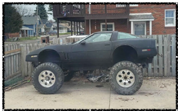
This customized 1987 Corvette 4x4 offered for sale on Facebook Marketplace for $10K is sitting on Chevy Blazer frame with 44-inch tall tires. Continue reading Corvette for Sale: 1987 Corvette 4x4 on Facebook Marketplace at Corvette: Sales, News & Lifestyle.
