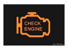
Whenever any of the monitored systems has an issue, the car's computer registers a "Trouble Code" that shows up on your dash as the dreaded "Check Engine Light". Unfortunately, this warning light tells the driver nothing. Without your own scan tool, you don't know if the problem is the engine, transmission, accidentavoidance system, or just a loose gas cap.
