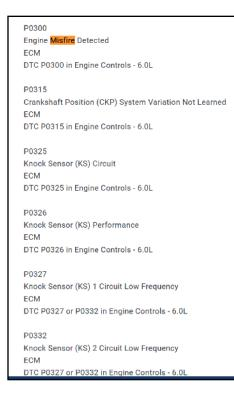
Codes prefixed with P pertain to the powertrain. Codes prefixed with B are related to the body. U codes indicate faults in the onboard network communications.
