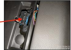
The OBD-2 scanner is plugged in. The scanner can be powered directly from the OBD connector, but most scanners also have batteries for use when disconnected. As soon as the scanner is connected to the OBD port, it will attempt to determine the type of mobile network that the car uses. There are five typcs of automotive networks that have been used. For all Corvettes, it is a CAN-II network.
